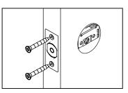
Insert latch and tighten screws.
