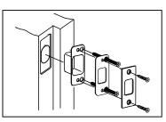
Install strike box and strike and tighten screws.
