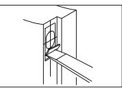
Measure one half of door thickness from door stop and vertically mark center line of strike. Drill aperture which is same with strike box 1-9/64" (29mm) deep at inter section of horizontal and vertical center line of strike. Match screw hole on strike with center lines on jamb. Mark outline and chisel 9/32" (7mm) deep for strike.
