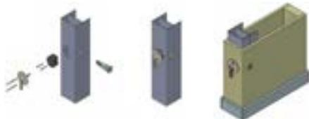
A. (above) requires a 2-1/8" bore through first stud to allow installation on second stud. For B. and C. (below), install bracket on first stud.
