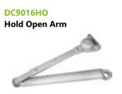
Non-handed arm with adjustable round slide arm for a wide range of frame conditions. Open to desired range, then tighten screw and lock nut: the door will hold in that position every time until changed. For parallel mount use parallel arm bracket
