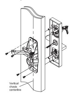
1. Attach escutcheon case to the door, thru-bolting the four (4) screws to the chassis, aligning spindle to hub of chassis.
