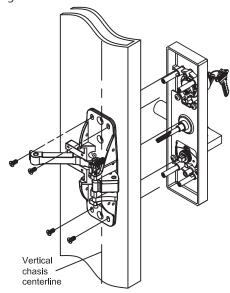
1. Attach escutcheon case to the door, thru-bolting the four (4) screws to the chassis, aligning spindle to hub of chassis.
