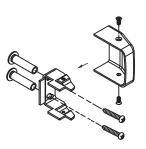
ATTACH END CAP TO MOUNTING PLATE WITH (2) COVER SCREWS.
