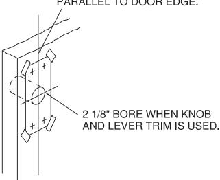
For doors without bore prep, mark vertical  $\Phi$  and horizontal  $\Phi$ chassis using the dimensions below.
