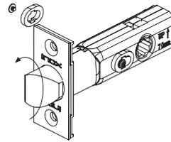
Determine door handing for latch and remove INSIDE washer (privacy pin side). Change the latch direction and faceplate (together) 180°.
