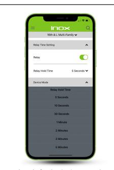
The default timing on the closing circuits is 5 seconds. In the Smart Mode, this timing is adjustable from 5 seconds to 5 minutes using the Smart APP in Device Settings.
