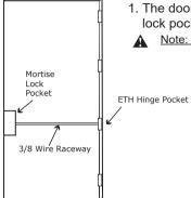
1. The door must be machined with a 3/8" wire raceway mortise lock pocket & prepped for an energy transfer hinge.
