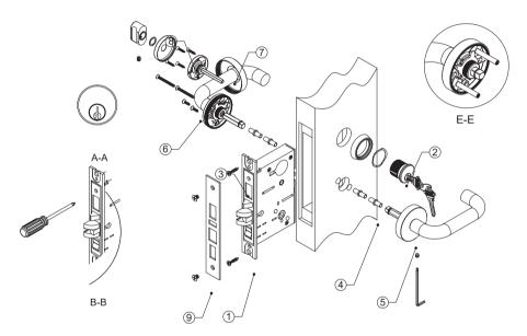
6. Install inside lever with 2 EA M4x35mm machine screws. And install 2EA #8x3/4" wood screws (for wood door)/self drilling screws (for metal door) for XRA/XSE rose. Then tightening the set screw using Allen key. See Section F-F
