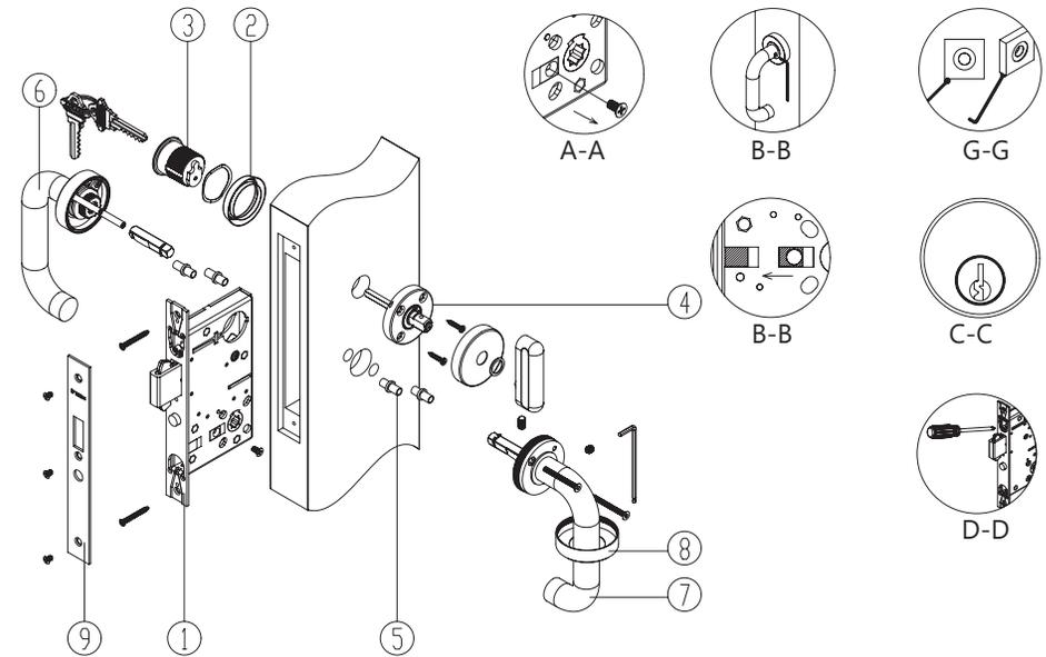
1. Install mortise lockcase in door prep. **NOTE:** DO NOT tighten the faceplate screws until the cylinder has been installed. Make sure the handing screws from the escaping side of the lockcase has been removed. See Section A-A. **NOTE:** Make sure the Entry locking block has been set to the B-B end direction.
