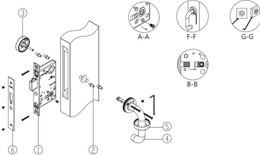
1. Install mortise lockcase in door prep. **NOTE:** DO NOT tighten the faceplate screws until the cylinder has been installed. Make sure handing screws from the escaping sides of the lockcase has been removed. See Section A-A. **NOTE:** Make sure the Entry locking block has been set to the B-B end direction.
