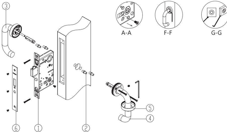
1. Install mortise lockcase in door prep. **NOTE:** Make sure handing screws from both sides of the lockcase has been removed. See Section A-A.
