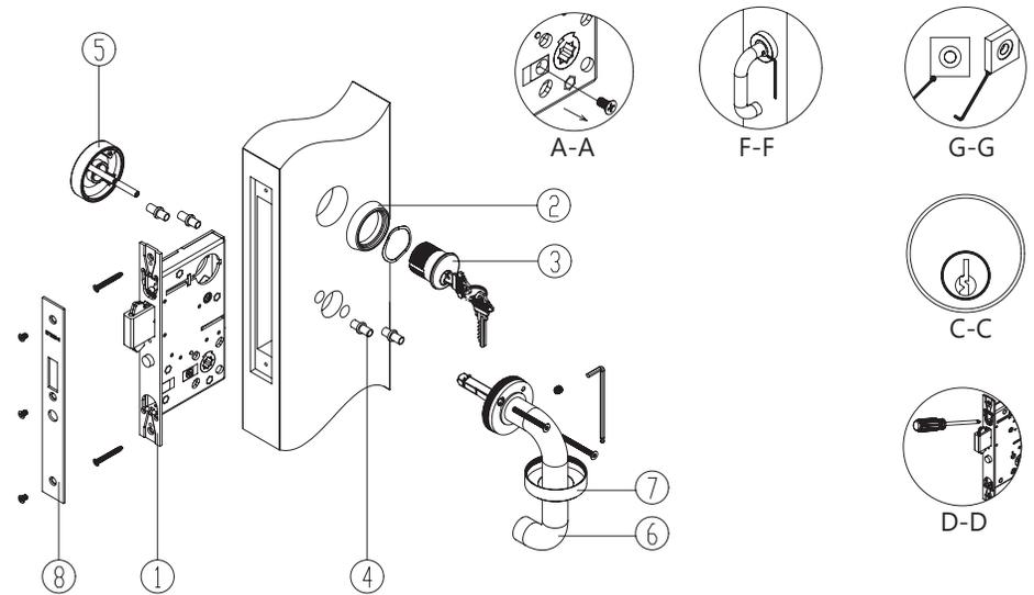
1. Install mortise lockcase in door prep. **NOTE:** DO NOT tighten the faceplate screws until the cylinder has been installed. Make sure handing screws from both sides of the lockcase has been removed. See Section A-A. **NOTE:** Make sure the Entry locking block has been set to the B-B end direction.
