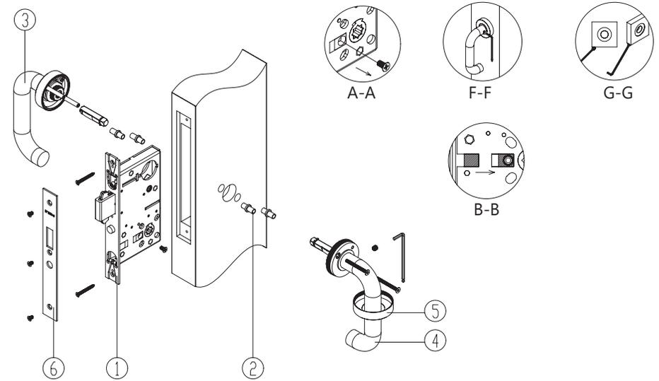
1. Install mortise lockcase in door prep. **NOTE:** DO NOT tighten the faceplate screws until the cylinder has been installed. Make sure handing screws from the escaping side of the lockcase has been removed. See Section A-A. **NOTE:** Make sure the Entry locking block has been set to the B-B end direction.
