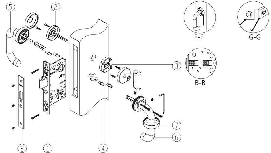
1. Install mortise lockcase in door prep. **NOTE:** Make sure the Entry locking block has been set to the B-B end direction.
