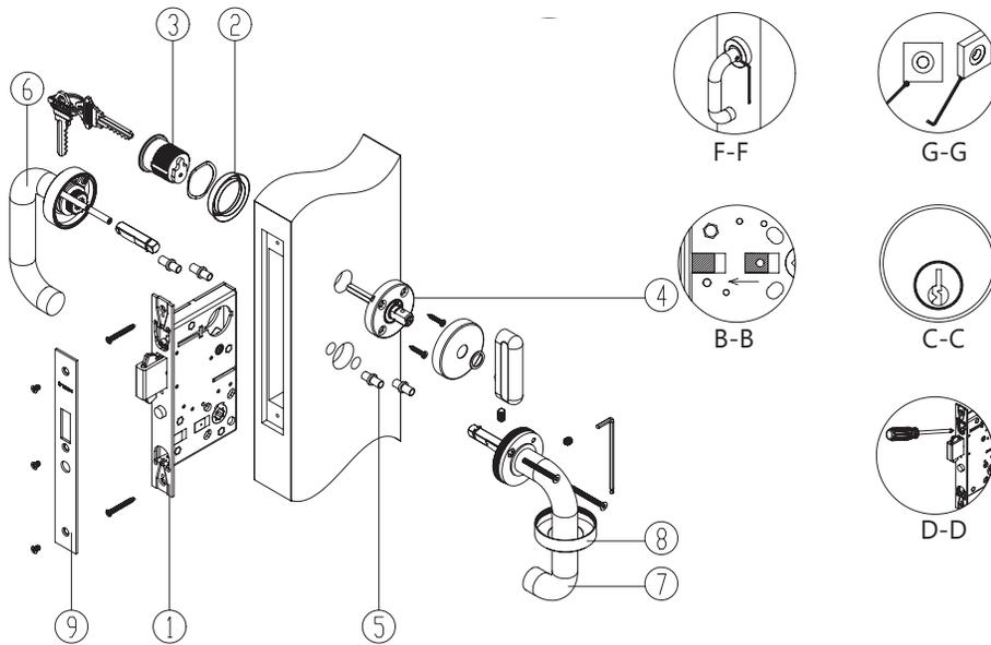
1. Install mortise lockcase in door prep. **NOTE:** DO NOT tighten the faceplate screws until the cylinder has been installed. **NOTE:** Make sure the Entry locking block has been set to the B-B end direction.
