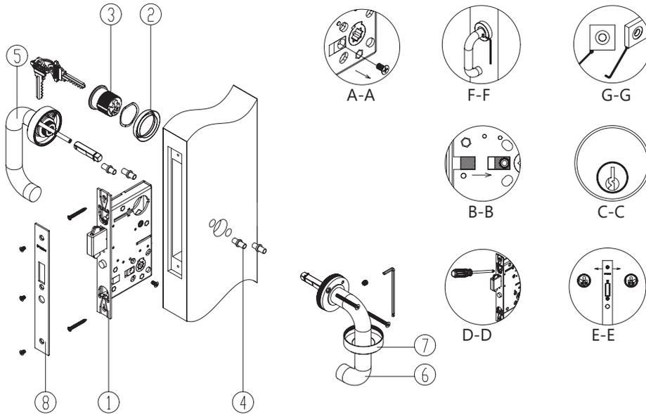
1. Install mortise lockcase in door prep. **NOTE:** DO NOT tighten the faceplate screws until the cylinder has been installed. Make sure handing screws from the escaping side of the lockcase has been removed. See Section A-A. **NOTE:** Make sure the Entry locking block has been set to the B-B end direction.
